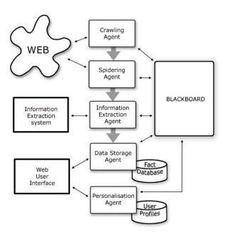
Figure 1: Architecture of the CROSSMARC system
